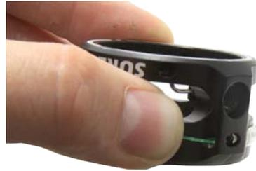
12. Put top fiber cover back on by inserting the ends of the fiber cover into the routing holes push to secure. **Ensure fiber is routed properly so it doesn't get pinched in this step.**
