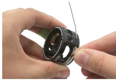
11. Insert fiber into the opposite fiber routing hole.
